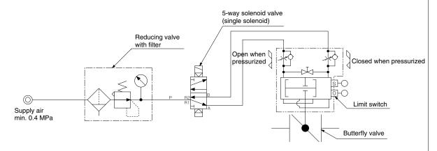
3 Butterfly valve closes when SOL.1 is energized. Butterfly valve opens when SOL.2 is energized.
